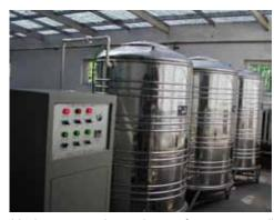
block structure, the equipment features a small footprint, offers greater flexibility than civil construction, is easy to install and use. The whole set of equipment adopts automatic control, low-power consumption design, can run automatically according to the water volume and shut down automatically when there is no wastewater.
